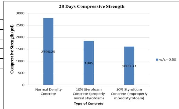
**Fig 2.** Effect of mixing procedure on compressive strength
