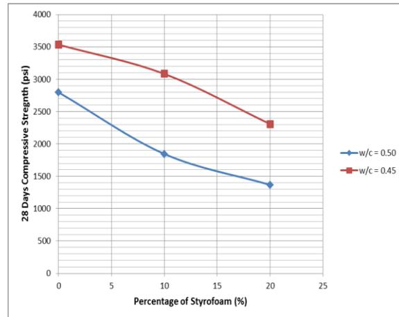
**Fig 3.** Effect of water-cement ratio
