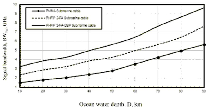
Figure 1. Transmitted signal bandwidth in relation to ocean water depth for different polymeric materials based submarine fiber cable system at the assumed set of the operating parameters.
