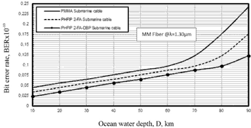
Figure 11. Bit error rate in relation to ocean water depth for different polymeric materials based submarine fiber cable system at the assumed set of the operating parameters.
