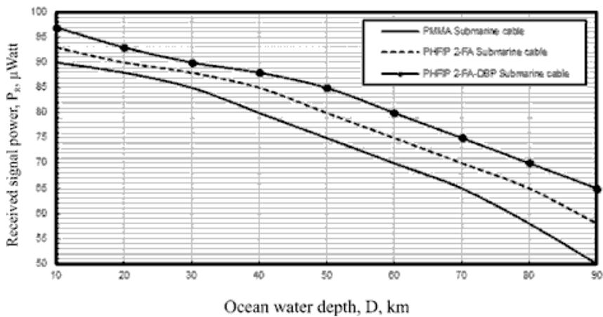
Figure 6. Signal transmission quality in relation to ocean water depth for different polymeric materials based submarine fiber cable system at the assumed set of the operating parameters.
