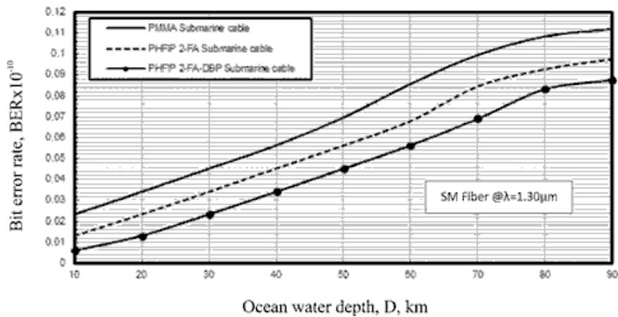
Figure 12. Bit error rate in relation to ocean water depth for different polymeric materials based submarine fiber cable system at the assumed set of the operating parameters.
