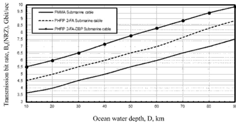
Figure 14. Transmission bit rates in relation to ocean water depth for different polymeric materials based submarine fiber cable system at the assumed set of the operating parameters.
