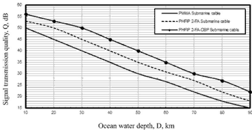
Figure 9. Signal transmission quality in relation to ocean water depth for different polymeric materials based submarine fiber cable system at the assumed set of the operating parameters.
