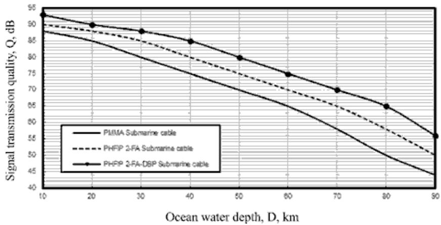
Figure 8. Signal transmission quality in relation to ocean water depth for different polymeric materials based submarine fiber cable system at the assumed set of the operating parameters.
