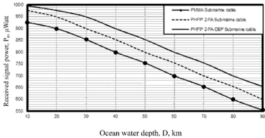
Figure 2. Received signal power in relation to ocean water depth for different polymeric materials based submarine fiber cable system at the assumed set of the operating parameters.
