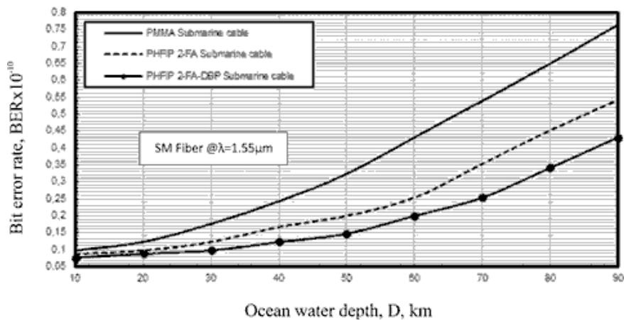
Figure 13. Bit error rate in relation to ocean water depth for different polymeric materials based submarine fiber cable system at the assumed set of the operating parameters.
