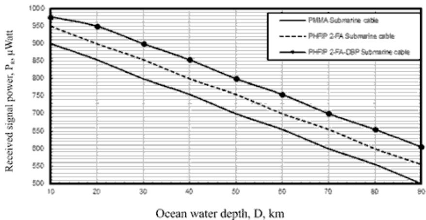
Figure 4. Received signal power in relation to ocean water depth for different polymeric materials based submarine fiber cable system at the assumed set of the operating parameters.
