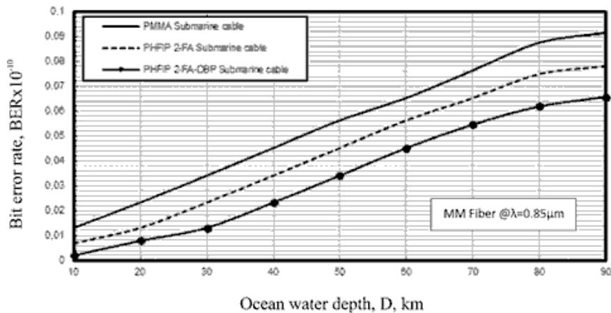
Figure 10. Bit error rate in relation to ocean water depth for different polymeric materials based submarine fiber cable system at the assumed set of the operating parameters.
