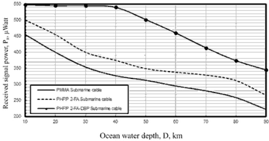
Figure 5. Received signal power in relation to ocean water depth for different polymeric materials based submarine fiber cable system at the assumed set of the operating parameters.
