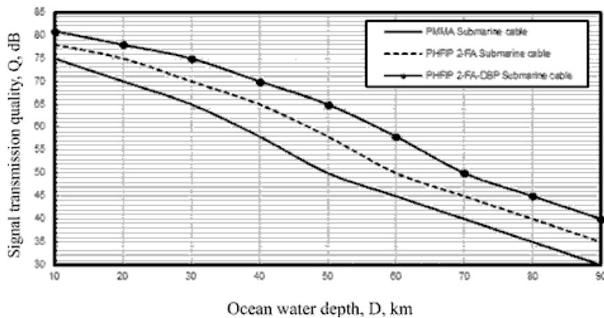
Figure 7. Signal transmission quality in relation to ocean water depth for different polymeric materials based submarine fiber cable system at the assumed set of the operating parameters.
