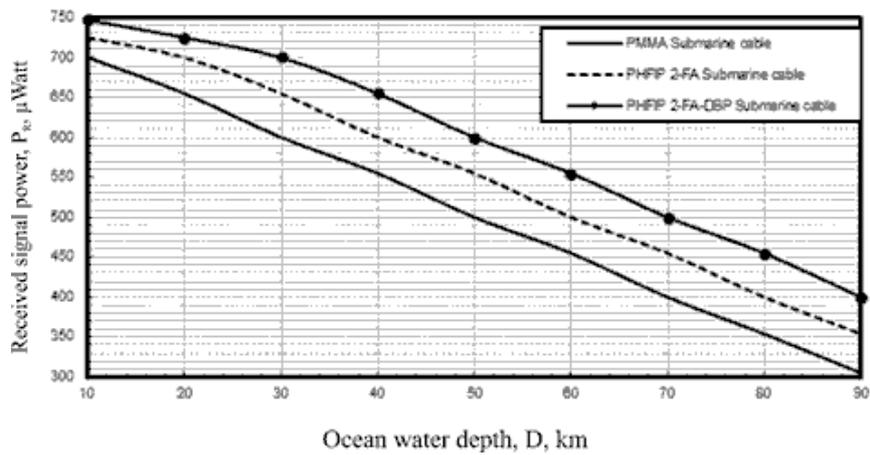
Figure 3. Received signal power in relation to ocean water depth for different polymeric materials based submarine fiber cable system at the assumed set of the operating parameters.
