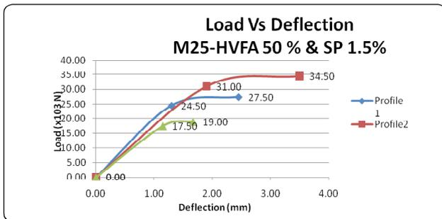
Fig. 4: Load vs. deflection curve-50% fly ash and 1.5 % sp.
