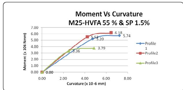
Fig. 8: Moment vs. curvature-55% fly ash and 1.5% sp.
