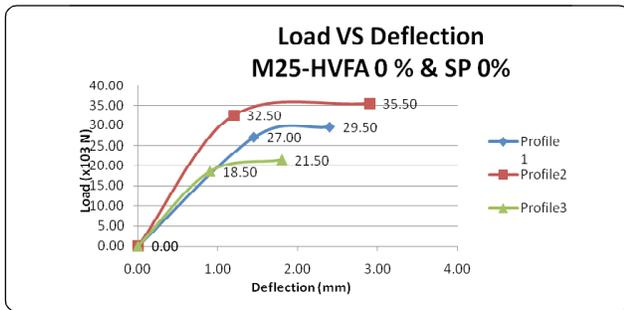
Fig. 3: Load vs. deflection curve-opcc.
