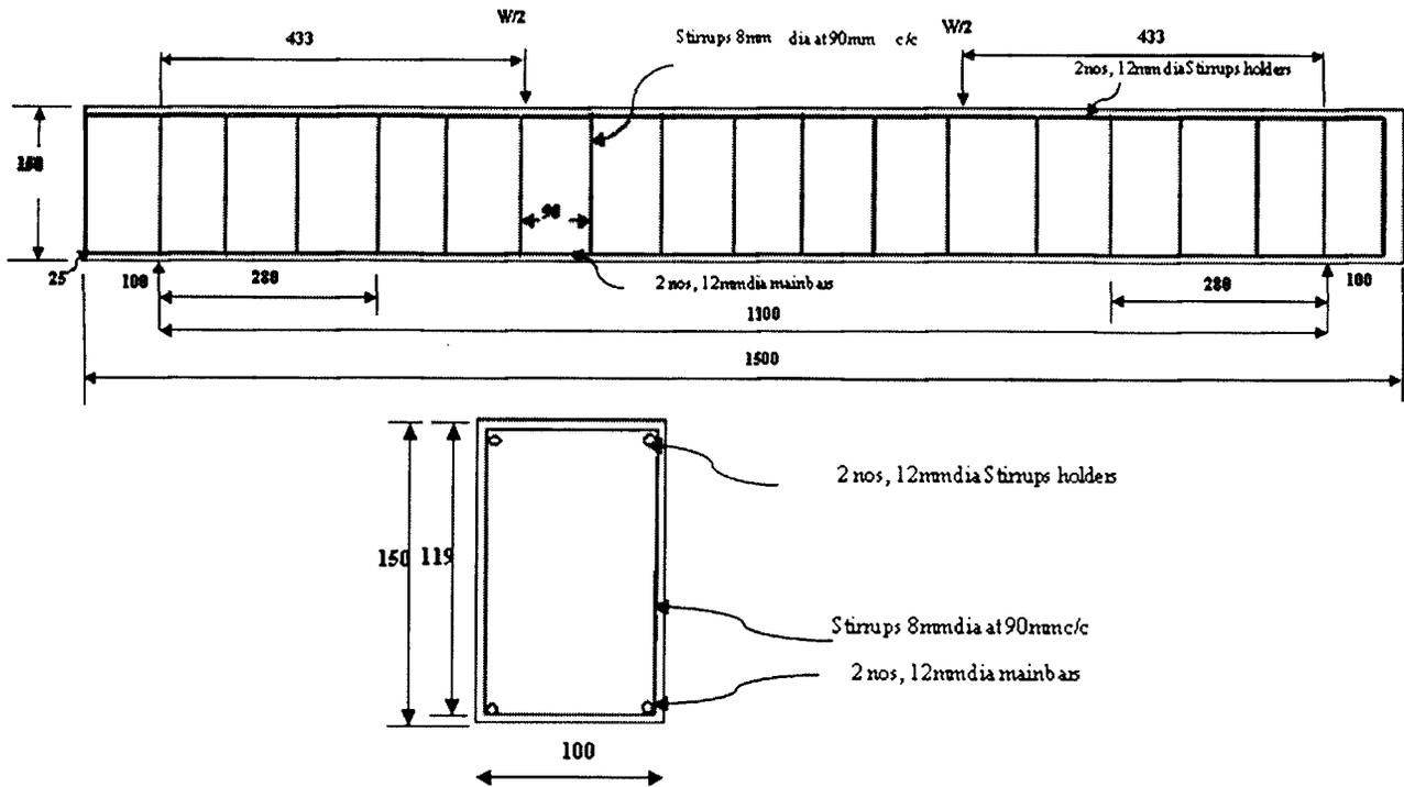
Fig. 1: Sectional details of non confinement of RC beam (profile-1, spacing,  $s = 0.75d$ ).
