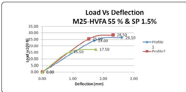
Fig. 5: Load vs. deflection curve-55% fly ash and 1.5% sp.
