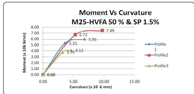
Fig. 7: Moment vs. curvature-50% fly ash and 1.5% sp.
