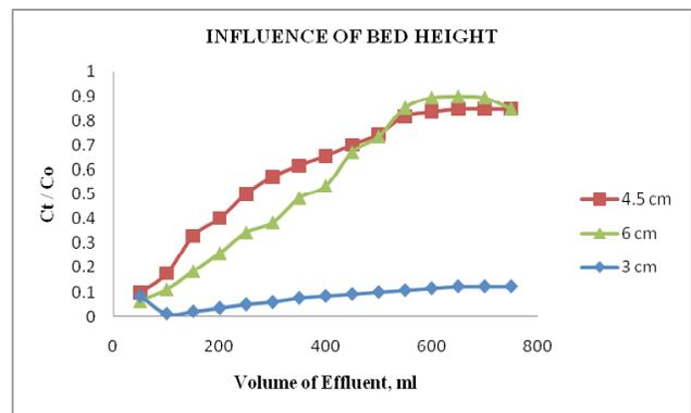
Fig. 4: Volume of the effluent Vs  $C_t/C_o$ .
