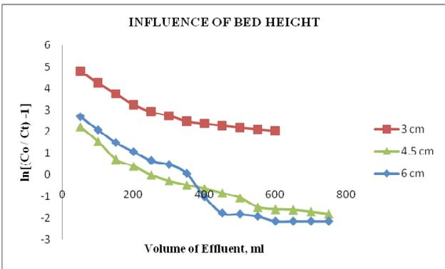
Fig. 5: Volume of the effluent Vs  $\ln(C_o/C_t - 1)$ .
