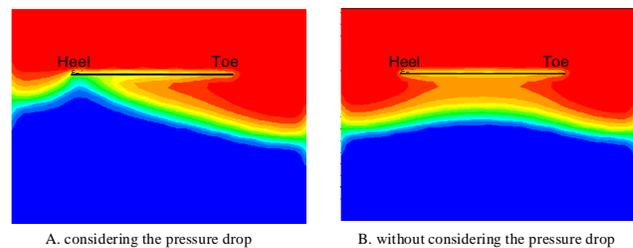
Fig. 2: The effect of pressure drop on remaining oil distribution.
