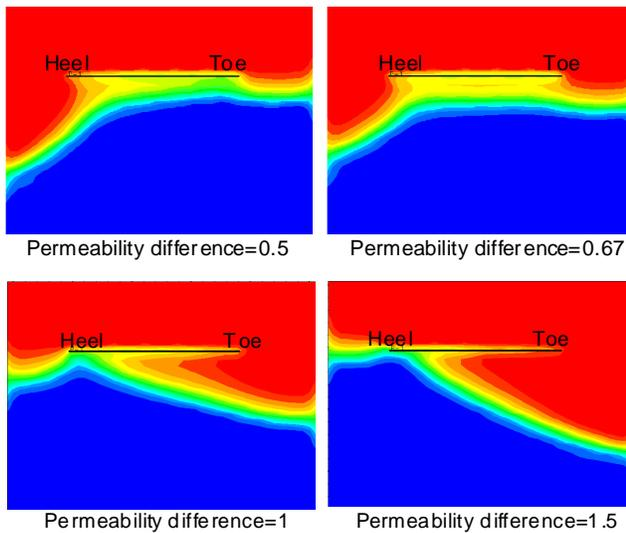
Fig. 3: The remaining oil distribution in different permeability difference.
