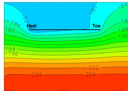
Fig. 1: The formation pressure distribution considering the pressure drop in the well bore.
