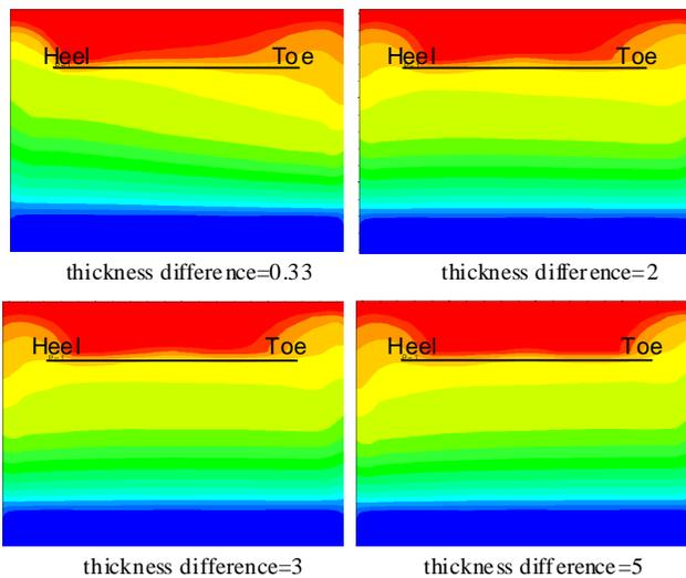
Fig. 4: The remaining oil distribution in different thickness difference.
