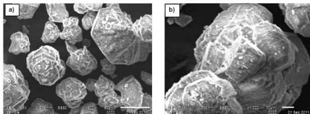
Fig. 2: Scanning electron micrographs of PAC: a) 500X, b) 1000X.
