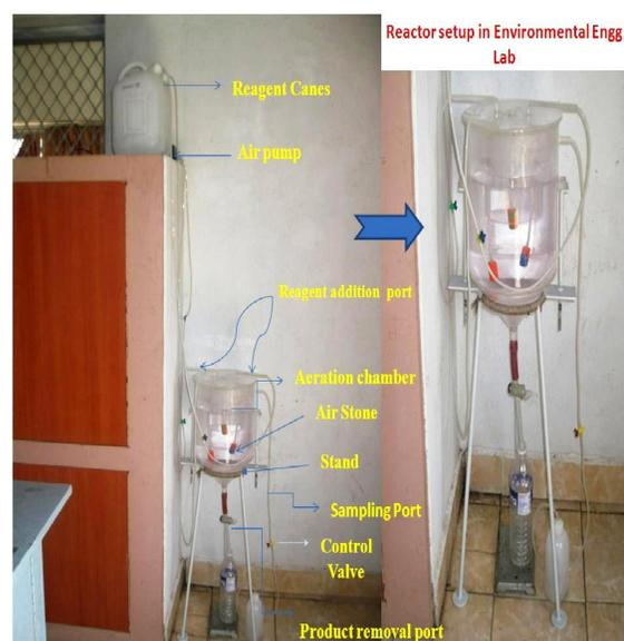
Fig. 1: Reactor setup.
