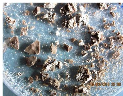
Fig. 3: Struvite crystal formed over the sludge of mixed wastewater with parent seed.
