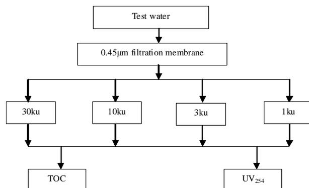
Fig. 1: Determining process of MV distribution of organic matters.
