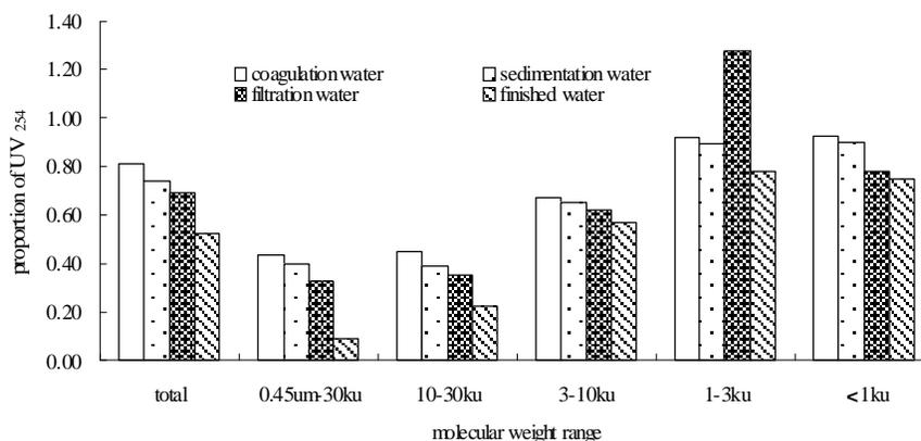
Fig. 8: The organic matter removal of the water of northern Ganjiang River on MV distribution of UV<sub>254</sub>.
