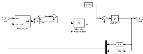
Figure 5: Simulation Diagram of the Phase Locked Loop
