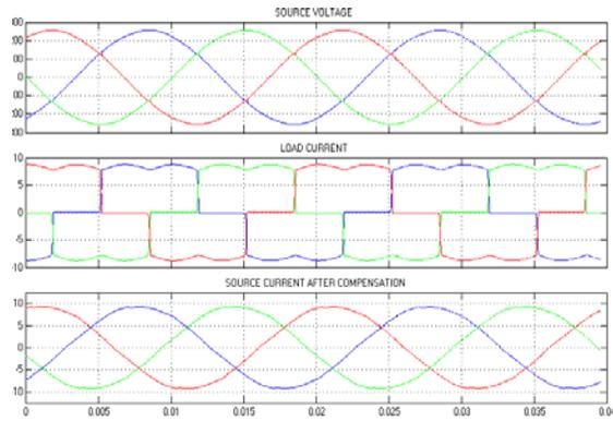
Figure 9: Source Voltage, Load Current and Source Current after Compensation
