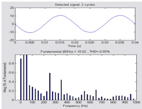
Figure 16: THD Plot for Balanced Case
