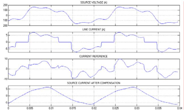
Figure 13: Source Voltage, Line Current, Current Reference and Source Current after Compensation for Phase C
