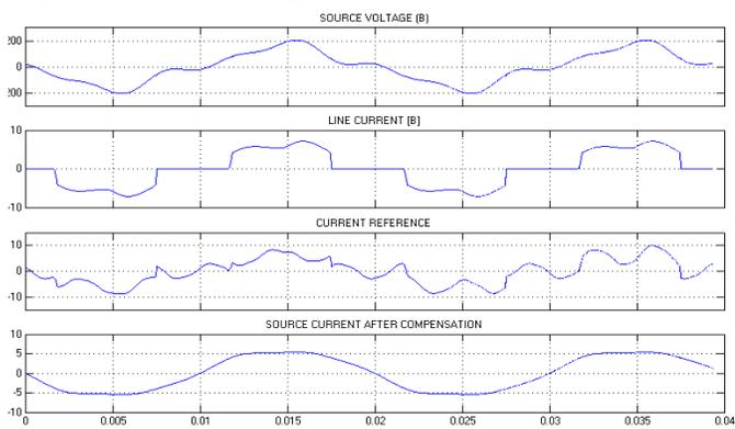
Figure 11: Source Voltage, Line Current, Current Reference and Source Current after Compensation for Phase A
