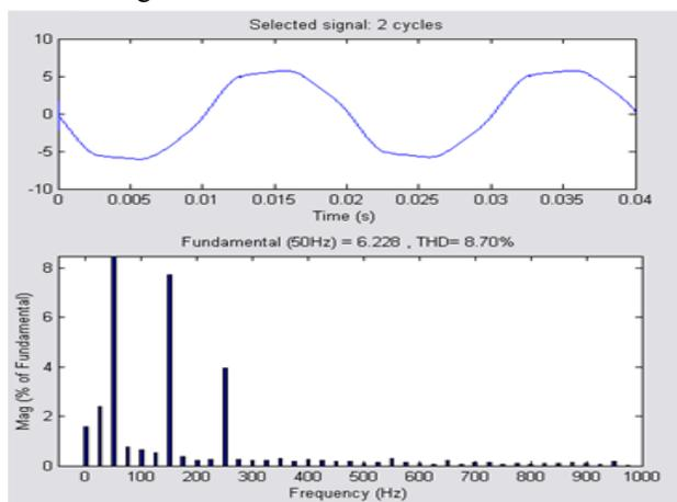
Figure 17: THD Plot for UN Balanced Case
