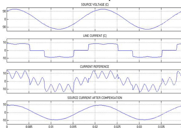
Figure 8: Source Voltage, Line Current, Current Reference and Source Current after Compensation for Phase c
