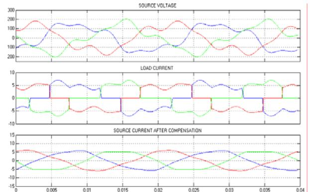
Figure 15: Source Voltage, Load Current and Source Current after Compensation
