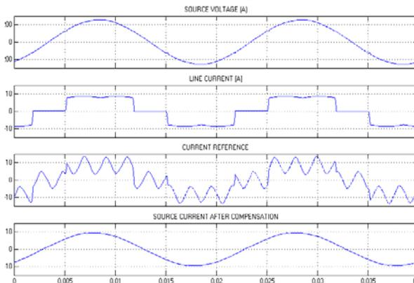
Figure 7: Source Voltage, Line Current, Current Reference and Source Current after Compensation for Phase B
