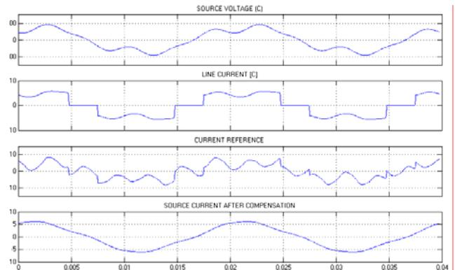
Figure 12: Source Voltage, Line Current, Current Reference and Source Current after Compensation for Phase B
