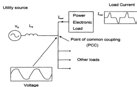
Figure 1: Harmonic Distortion at PCC
